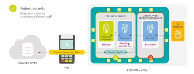
What happens in a microcontroller is vulnerable to manipulation. What happens in a secure element remains hidden and protected.
