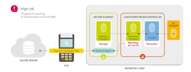
Using software security to protect matching is NEVER as secure as using hardware security.
