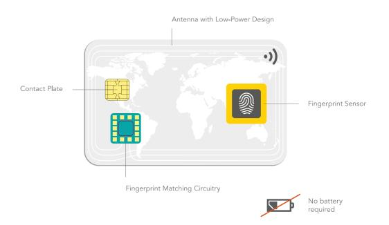
The thin, battery-free form factor is compatible with the current infrastructure
